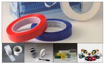
**EGP** is a low-density polyethylene tape which offers excellent chemical resistance and good conformability. Wound on a plastic core, the **EGP** tape has a strong tack and can be used for maintenance applications in place of masking and duct tapes. Inherently clean with low outgassing, the clean peel and reseal properties of the tape are a plus factor in controlled environments and cleanroom support applications. **EGP** is available in eight vibrant colors.
