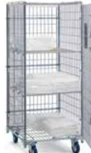
> MONOBLOC SECURITY ROLL ref: 4 495 72 97 Galvanized steel tube and wire. Permissible load: up to 500 kg. Rubber casters: ø 125 mm, 2 fixed + 2 swivelling. Capacity: 735 dm 3 . Available in 2 heights: 1700 and 1900 mm.
